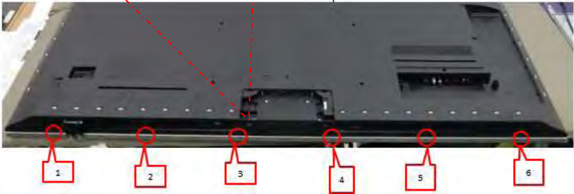
(65"/75" PML9636 rear cover removal-1)
